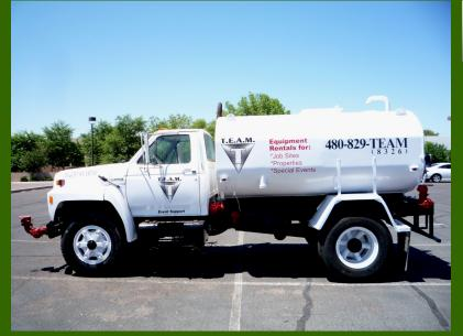
Our water trucks are utilized to fill our water barricades on site, as well as provide dust control for dirt parking lots and other open areas at special events, construction sites and other areas needing EPA dust control compliance or general dirt calming. We also can use both our water trucks and our pumper truck to cool crowds and bring large quantities of water to any area quickly. Our trucks can also pump out and remove water in case of monsoon storm or other flooding.
